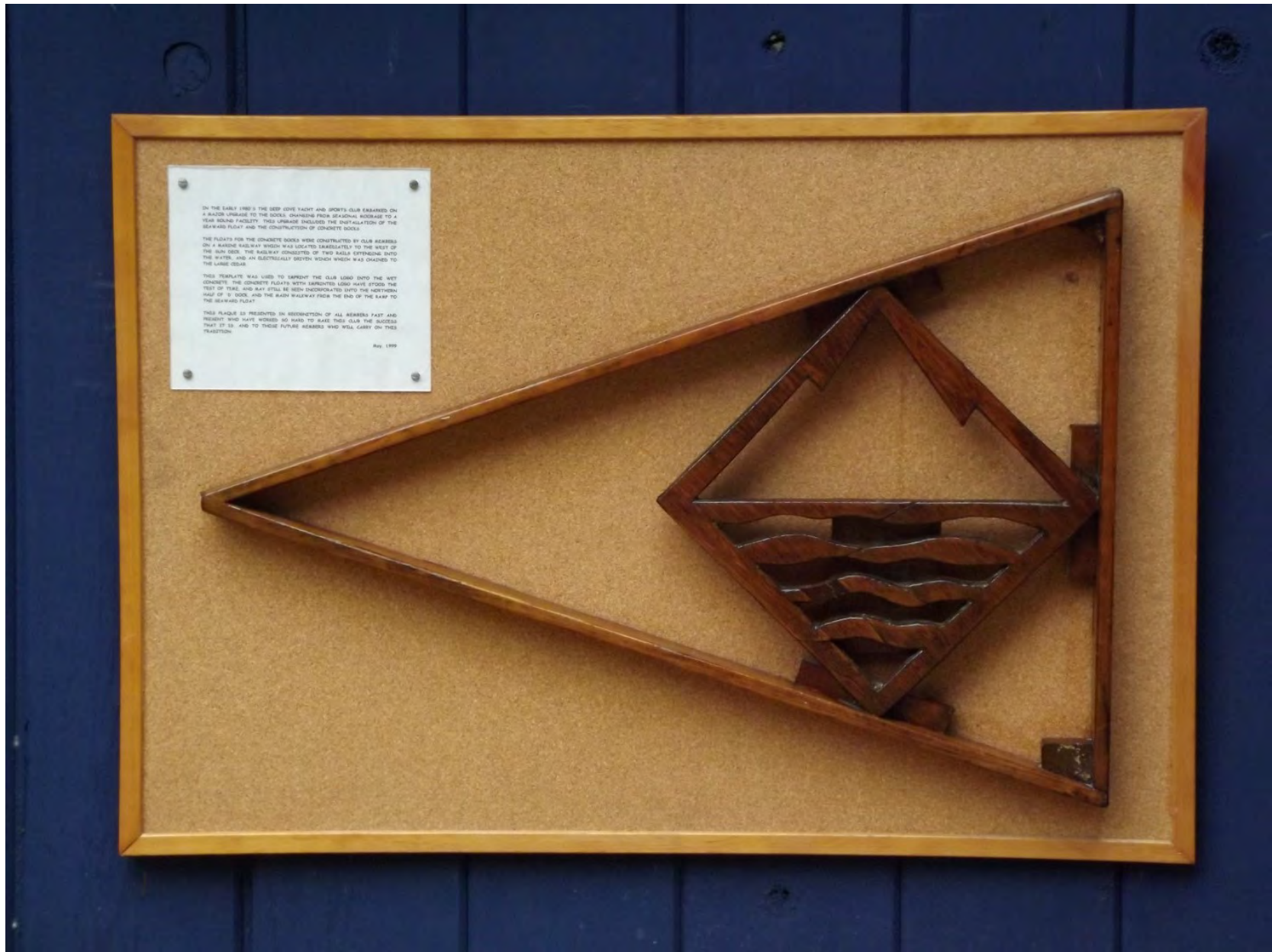
The template for embossing the concrete blocks – made by Horst Oetter and on display on the stairs to the basement.
